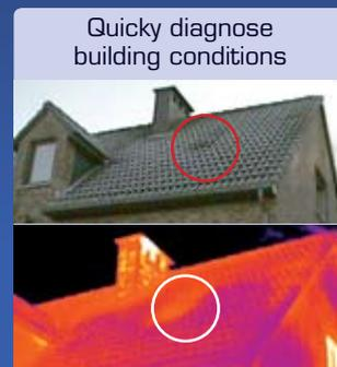
The infrared inspection locates missing insulation in the roof. This can now be repaired and further energy loss prevented.
